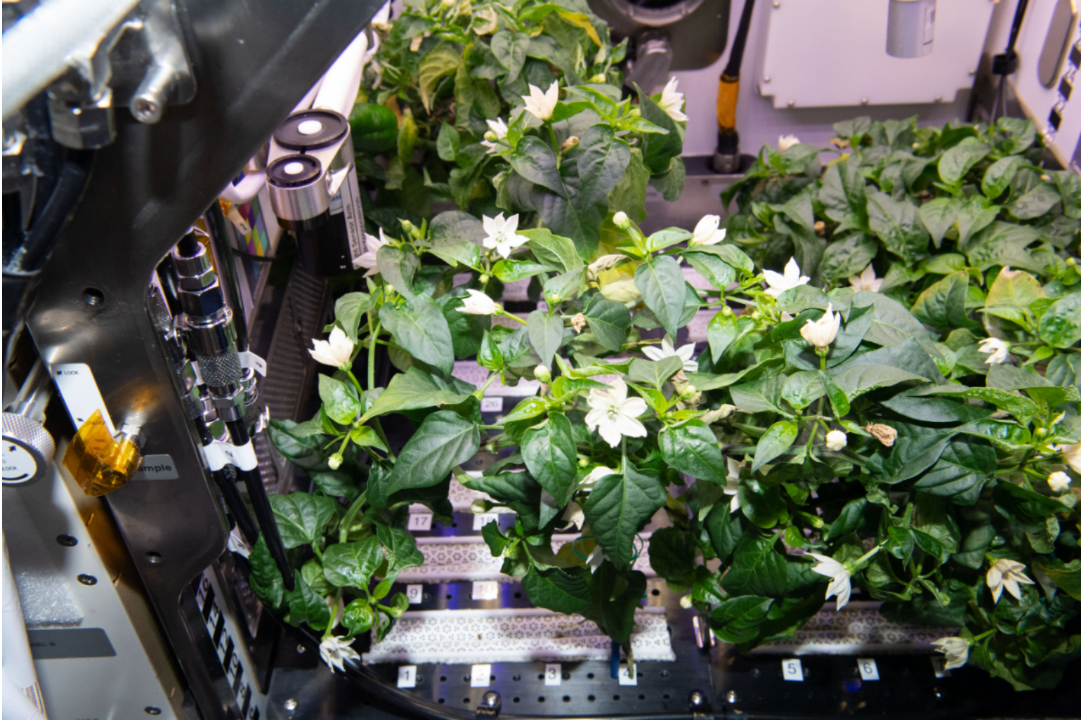
Hatch Green Chile plants are pictured growing in the Advanced Plant Habitat aboard the International Space Station (ISS). The Microgravity Growth of New Mexico Hatch Green Chile as a Technical Display of Advanced Plant Habitat's Capabilities (Plant Habitat-04) demonstrates using the Advanced Plant Habitat (APH) by growing peppers in space for the first time. Credit: NASA/JSC
