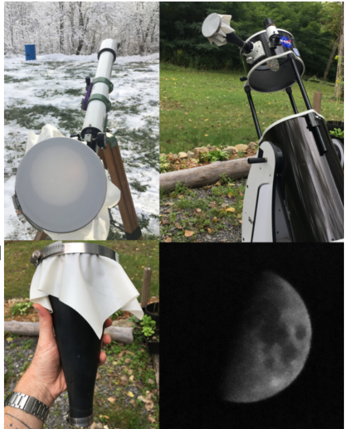
Sun Funnels in action! Starting clockwise from the bottom left, a standalone Sun Funnel; attached to a small refractor to observe the transit of Mercury in 2019; attached to a large telescope in preparation for evening lunar observing; projection of the Moon on a funnel from a medium-size scope (5 inches).
