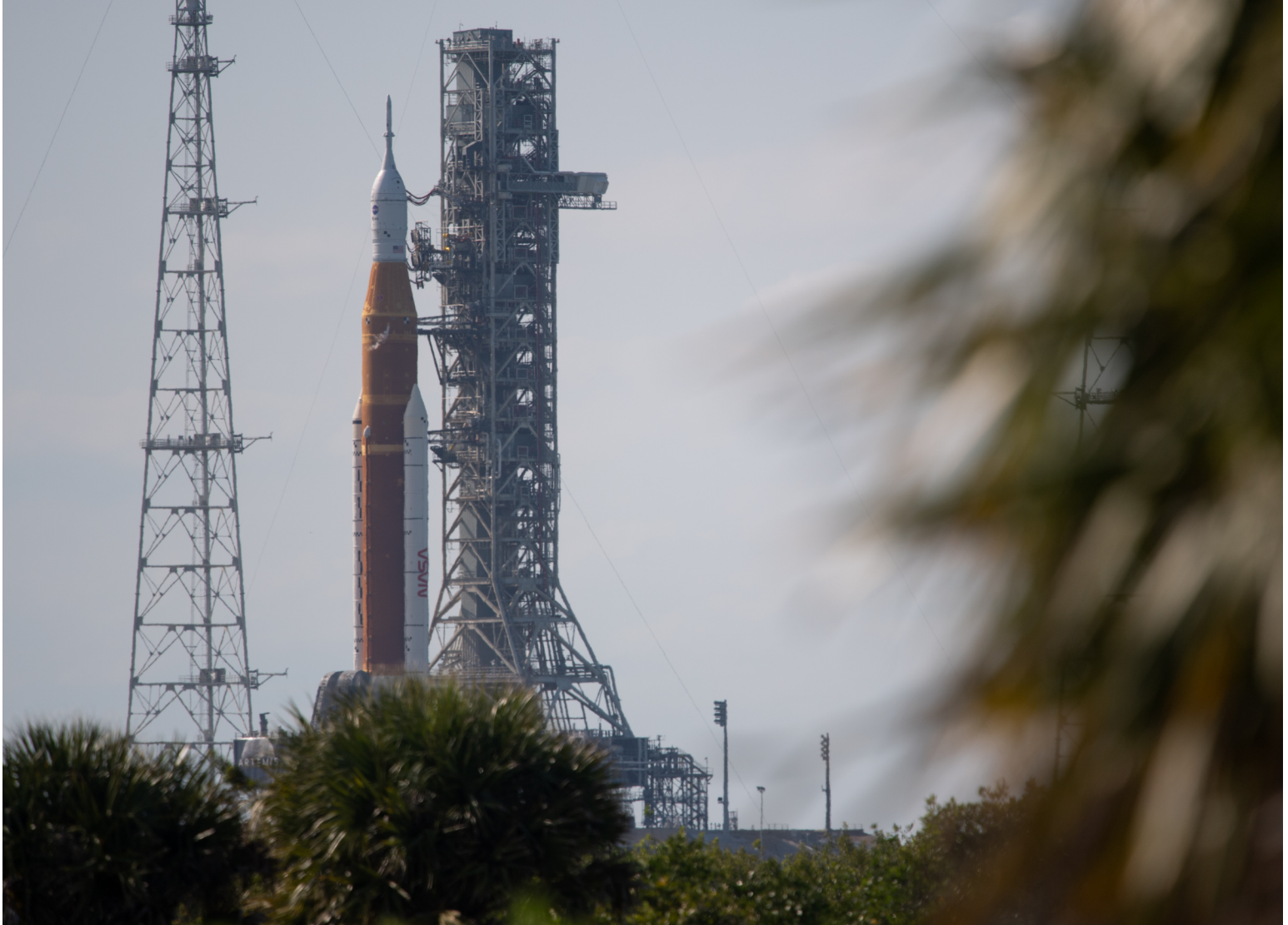
NASA's Space Launch System (SLS) rocket with the Orion spacecraft aboard is seen atop a mobile launcher at Launch Complex 39B, Monday, April 4, 2022, as the Artemis I launch team conducts the wet dress rehearsal test at NASA's Kennedy Space Center in Florida. Ahead of NASA's Artemis I flight test, the wet dress rehearsal will run the Artemis I launch team through operations to load propellant, conduct a full launch countdown, demonstrate the ability to recycle the countdown clock, and drain the tanks to practice timelines and procedures for launch. Photo Credit: (NASA/Joel Kowsky)
