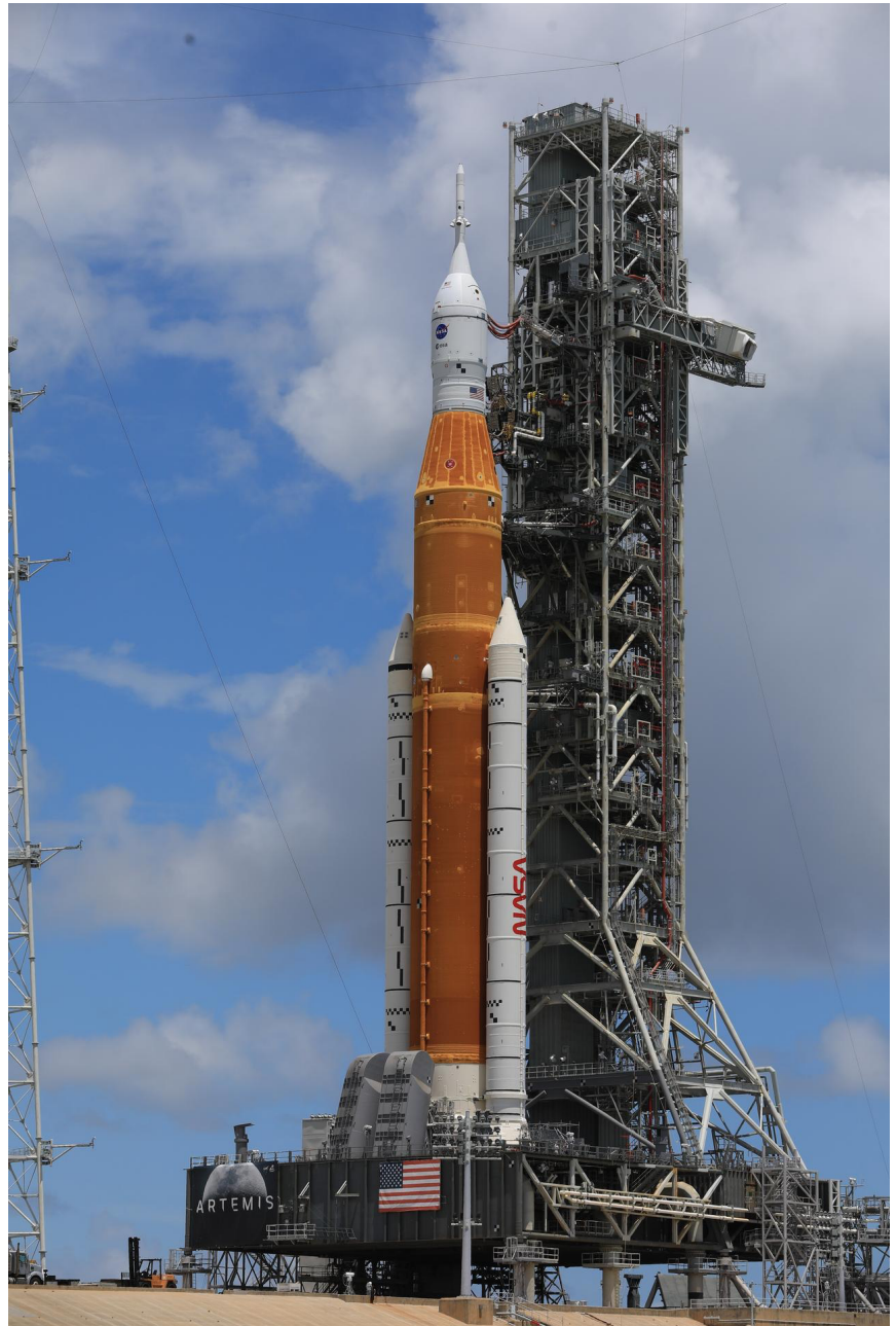
A view of the Artemis I Space Launch System (SLS) and Orion spacecraft atop the mobile launcher at Launch Pad 39B at NASA's Kennedy Space Center in Florida on June 30, 2022. The SLS and Orion were transported to the pad on crawler-transporter 2 for a prelaunch test called a wet dress rehearsal. NASA/Kim Shiflett
